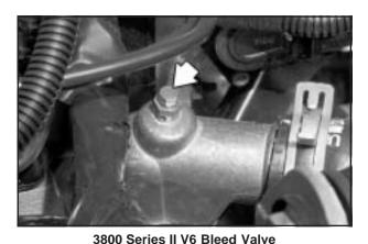
3800 V6 engine: There is one bleed valve. It is located on the thermostat housing.
